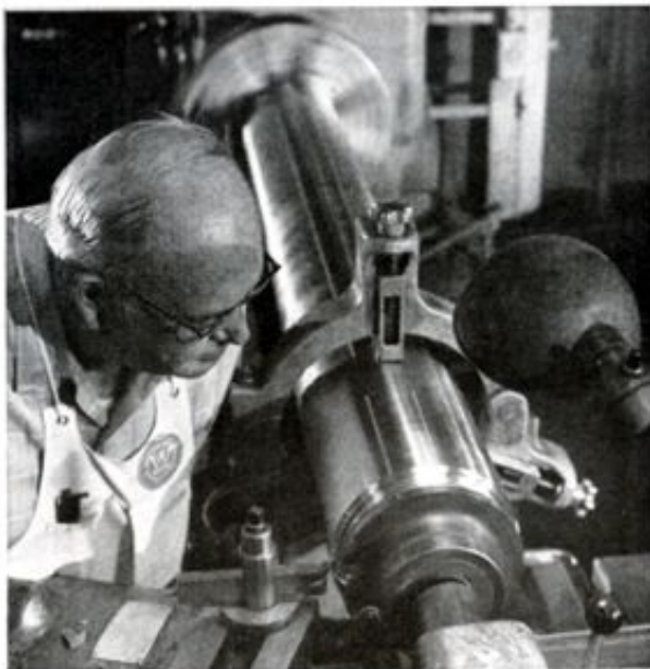
Veteran Westinghouse machinist Carl W. Buehrig machines to final shape the tubular body of the gleaming Time Capsule II. Machine work on the capsule was carried out at the East Pittsburgh plant of Westinghouse.
