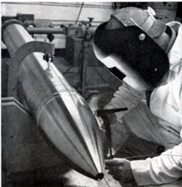
One of the bullet-shaped end pieces of Time Capsule II is welded into place at the East Pittsburgh plant of Westinghouse Electric Corporation. The capsule is made of Kromarc, a "super" stainless steel having unusual weldability.
