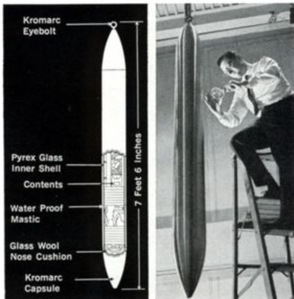
The diagram shows how Time Capsule II is constructed. The Kromarc stainless steel capsule contains a glass inner shell which will provide an air-tight envelope for the capsule contents. On the right, metallurgist H. D. Greenberg, who supervised construction of the new Time Capsule, gives the gleaming, torpedo-shaped structure its final check-out.
